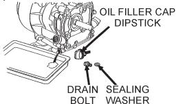
Figure 25. Engine Oil (Draining)
